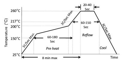
Figure 3. Solder Reflow Profile
