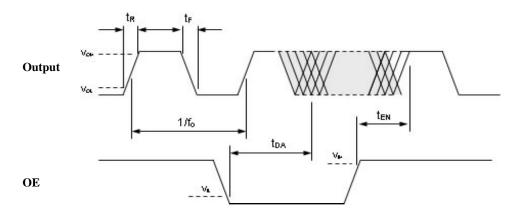
Figure 2. LVCMOS Output Waveform
