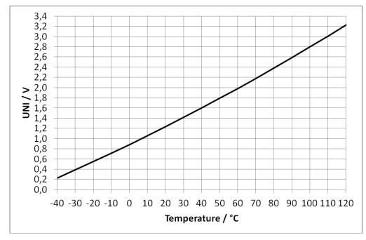
Output voltage characteristics with VCC = 3.3V
