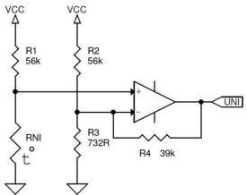
Example of analog interface circuit for high accuracy measurement using Ni1000SOT sensor
