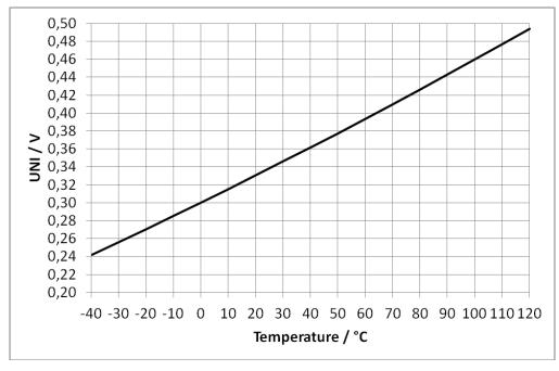
Output voltage characteristics with VCC = 3.3V
