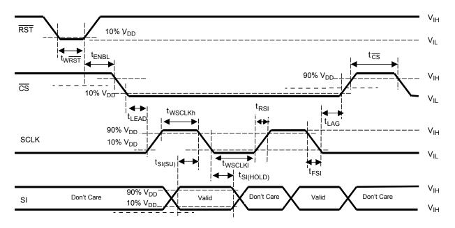
Figure 7. Input Timing Switching Characteristics
