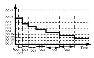
Figure 14. Overcurrent profile with OCHI bit set to '1'
