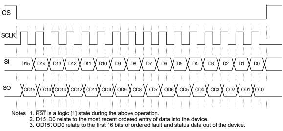
Figure 9. Single 16-Bit Word SPI Communication
