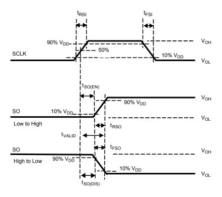
Figure 8. SCLK Waveform and Valid SO Data Delay Time
