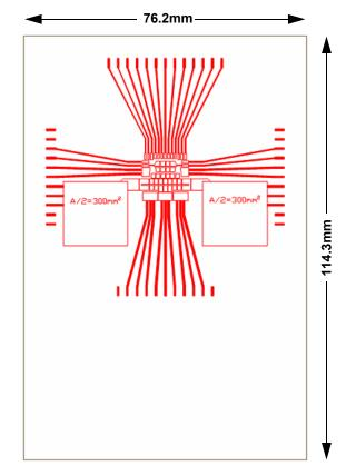
Figure 16. 1s JEDEC Thermal Test Board Layout
