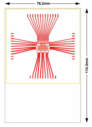
Figure 17. 2s2p JDEC Thermal Test Board (Red - Top Layer, Yellow - Two Buried Layers)
