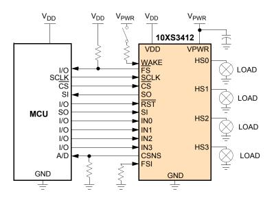
Figure 1. 10XS3412 Simplified Application Diagram
