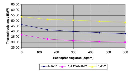
Figure 19. Steady State Thermal Resistance in Dependance on Heat Streading Area; 1s JEDEC Thermal Test Board with Spreading Areas
