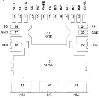
Figure 3. 10XS3412 Pin Connections
