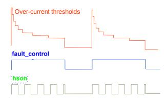
In steady state, the wire harness will be protected by OCLO2 current level by default. Three other DC overcurrent
