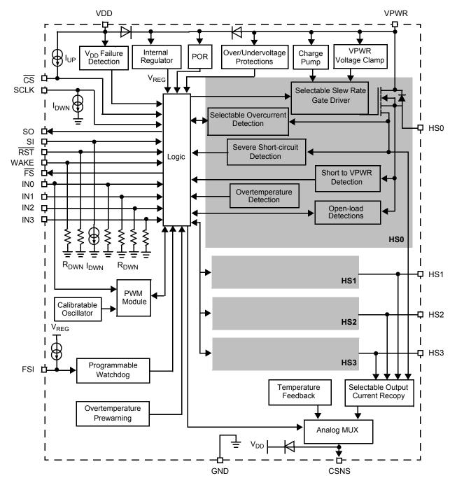
Figure 2. 10XS3412 Simplified Internal Block Diagram
