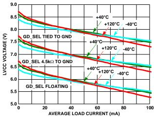
FIGURE 4. TYPICAL LVCC VARIATION WITH LOAD (DEM)
