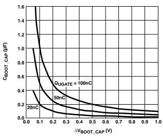
FIGURE 5. BOOTSTRAP CAPACITANCE vs BOOT RIPPLE VOLTAGE
