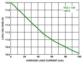
FIGURE 3. TYPICAL LVCC VARIATION WITH LOAD (CCM)
