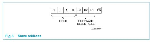
The next three significant bits of the slave address field (B3, B2, B1) are the block selection bits. It is used by the host to select one out of eight blocks (1 block = 256 bytes of memory). These are, in effect, the three most significant bits of the word address.
