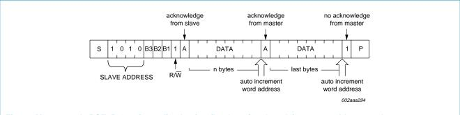
Fig 8. Master reads PCF85116-3 immediately after first byte (read mode); current address read.
