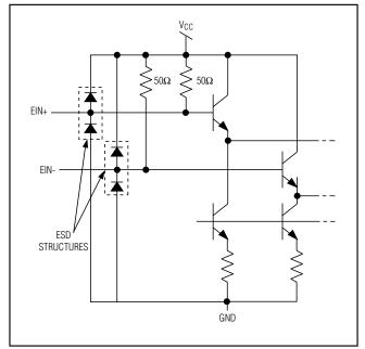
Figure 2. CML Input Equivalent Circuit
