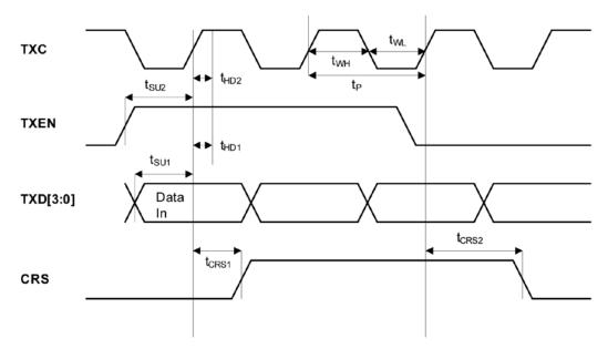
Figure 12. MII Transmit Timing (100Base-TX)
