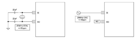
Figure 6. 25MHz Crystal/Oscillator Reference Clock
