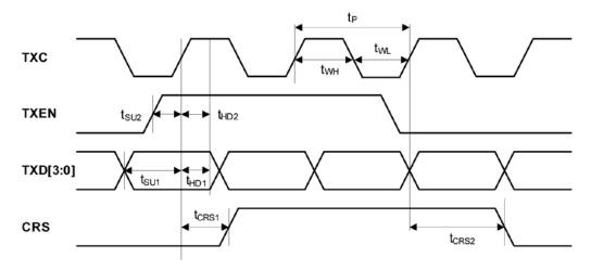
Figure 10. MII Transmit Timing (10Base-T)
