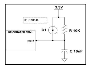
Figure 19. Recommended Reset Circuit
