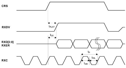
Figure 11. MII Receive Timing (10Base-T)
