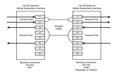
Figure 4. Typical Straight Cable Connection
