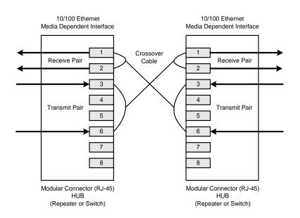
Figure 5. Typical Crossover Cable Connection
