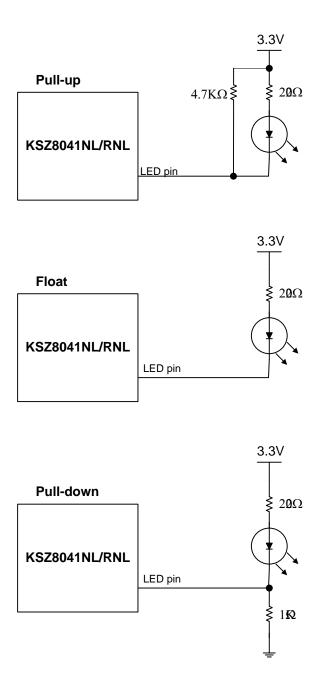
Figure 21. Reference Circuits for LED Strapping Pins
