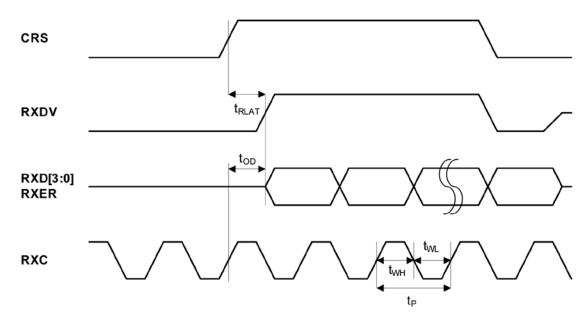
Figure 13. MII Receive Timing (100Base-TX)
