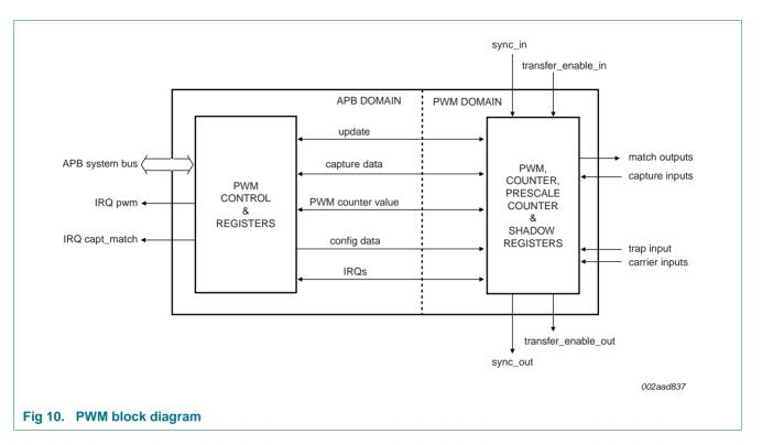
The PWM block diagram in Figure 10 shows the basic architecture of each PWM. PWM functionality is split into two major parts, a APB domain and a PWM domain, both of which run on clocks derived from the BASE\_MSCSS\_CLK. This split into two domains affects behavior from a system-level perspective. The actual PWM and prescale counters are located in the PWM domain but system control takes place in the APB domain.
