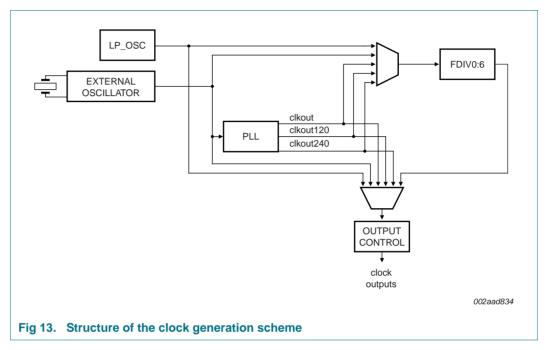
Any output generator (except for BASE\_SAFE\_CLK and BASE\_PCR\_CLK) can be connected to either a fractional divider (FDIV0:6) or to one of the outputs of the PLL or to LP\_OSC/crystal oscillator directly. BASE\_SAFE\_CLK and BASE\_PCR\_CLK can use only LP\_OSC as source.
