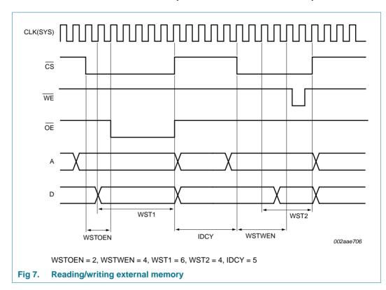
Usage of the idle/turn-around time (IDCY) is demonstrated In Figure 7. Extra wait states are added between a read and a write cycle in the same external memory device.
