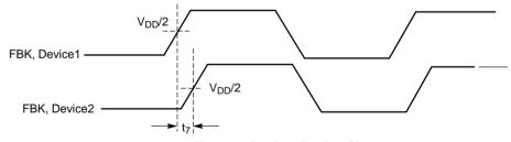
Figure 7. Device-Device Skew
