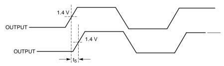
Figure 5. Output-Output Skew
