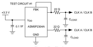
Figure 8. Test Circuit
