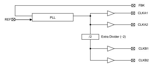
Figure 1. Block Diagram
