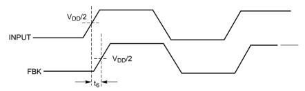
Figure 6. Input-Output Propagation Delay
